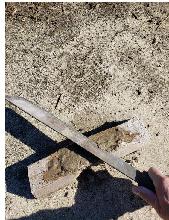
your blade across the "Sand Stick" Board and sharpen away. You may find applying some downward pressure to get the blade to bite into the board a bit may help, but you will need to develop a feel for what is right and works for you.
